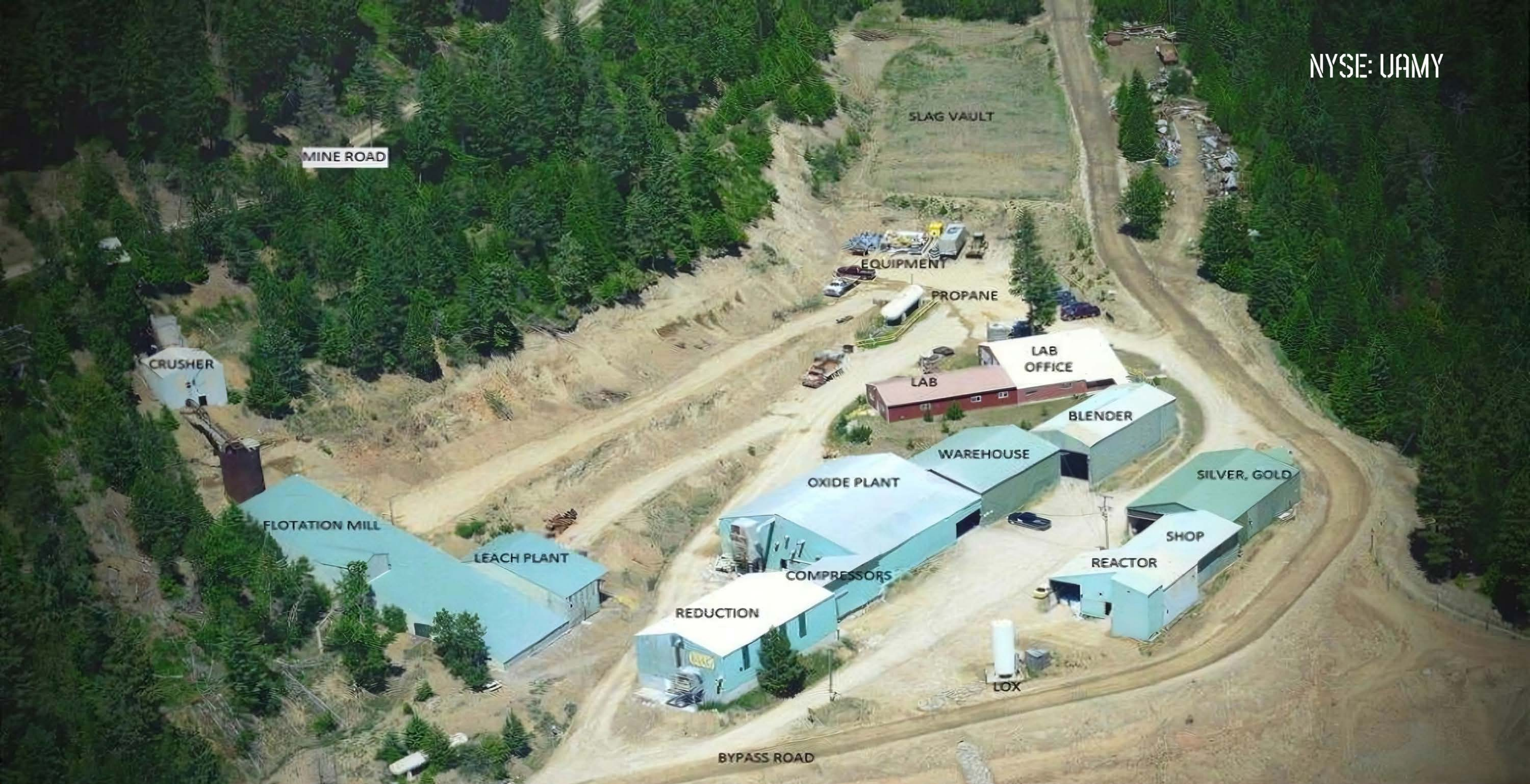
ANTIMONY SMELTER PLANT - THOMPSON FALLS, MONTANA NOTE: SMELTER CAPACITY OF 320 TONS PER MONTH OR 11 TONS PER DAY
